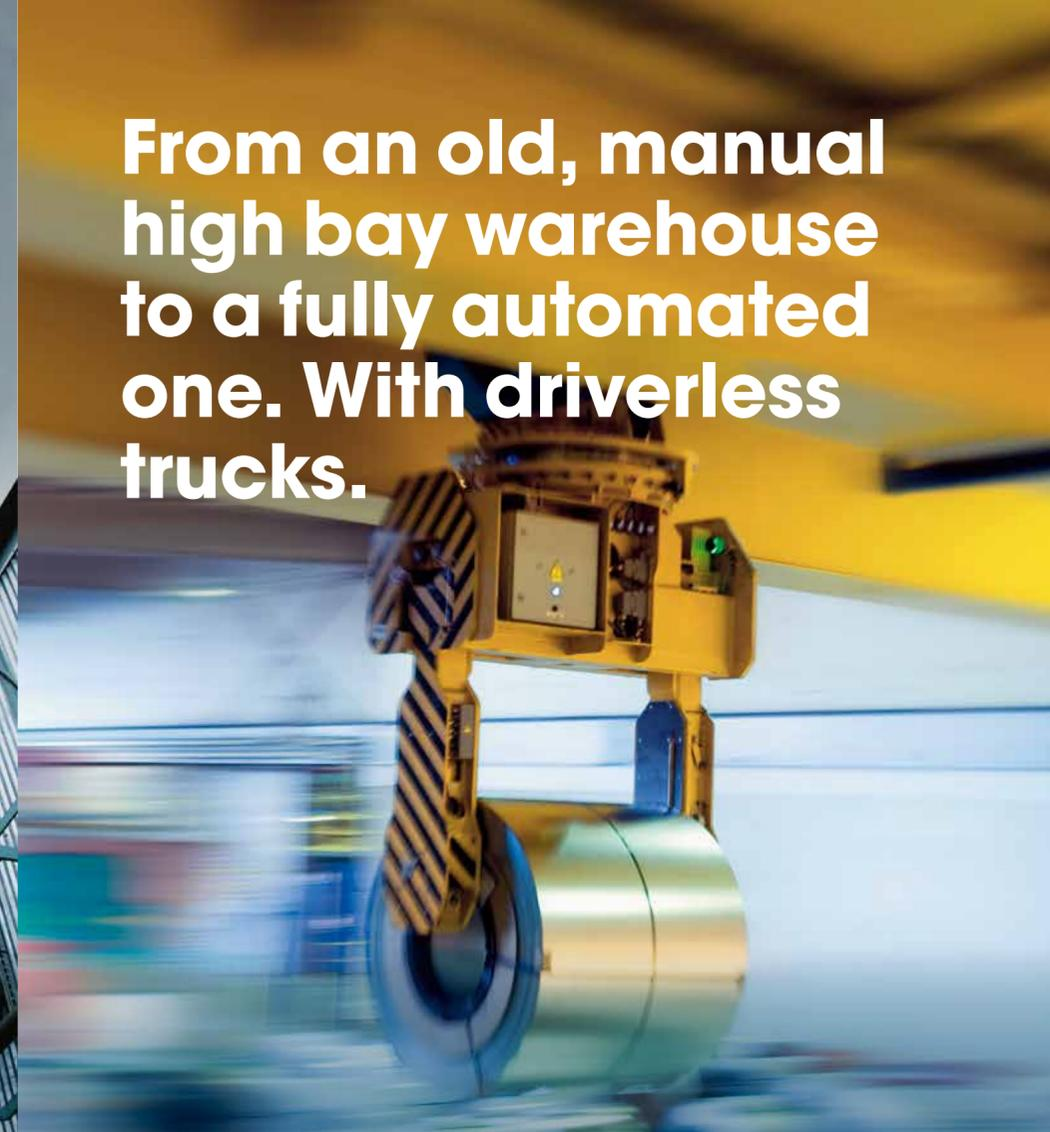
SSAB wanted to make their old high bay storage facility in Borlänge more efficient. Midroc Automation was given full responsibility for creating a fully automated warehouse in which four new overhead traveling cranes and one remodeled older one could be linked up in a new system with four coil trolleys and three automated trucks.
